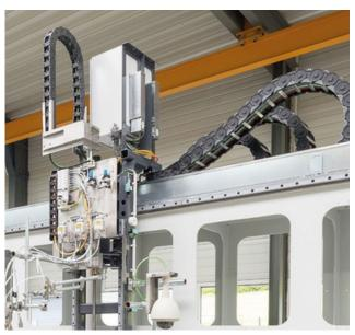
Drag chain systems are used for a wide range of applications and travel distances. HELUKABEL has the right solution for every application: from self-supporting drag chains for short distances to gliding drag chains for longer distances. Our range also includes special slide shoes to reduce wear and channel systems to guide the chains. Even for very long movement distances and high additional loads, the MARATHON system is a reliable solution
